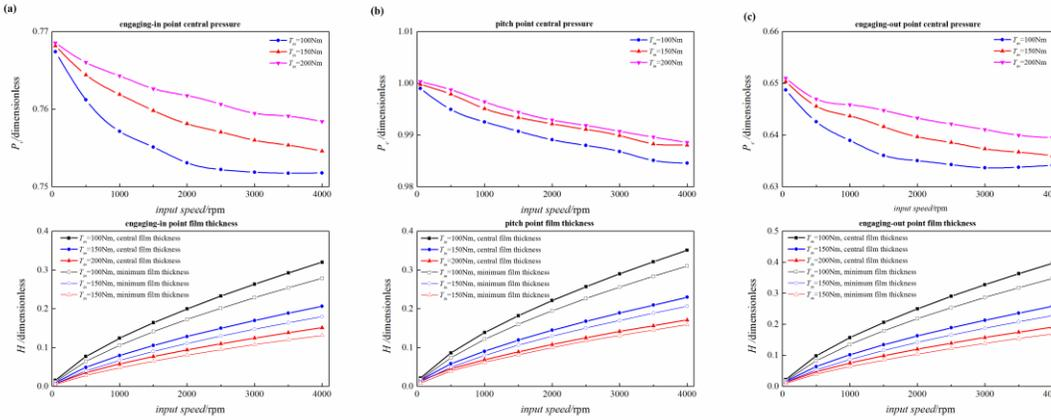
**Fig. 6.** Dimensionless central pressure and film thickness at (a) engaging-in point, (b) pitch point and (c) engaging-out point under different applied torques and operating speeds.
