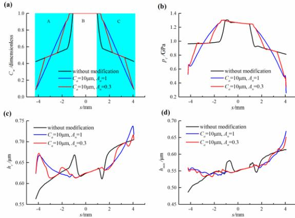
**Fig. 3.** Effects of tooth profile modification on: (a) gear tooth load, (b) central film pressure, (c) central film thickness and (d) minimum film thickness.
