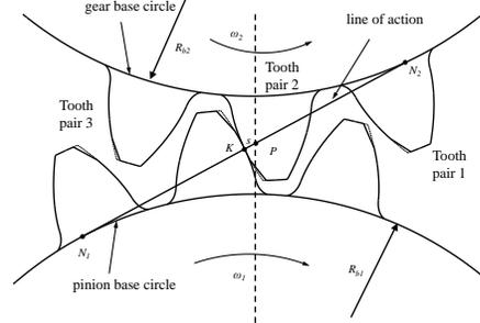
**Fig. 2.** diagram of a meshing gear pair
