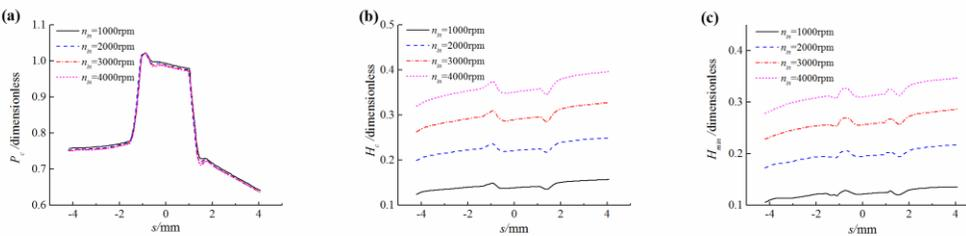
**Fig. 4.** Effects of operating speed on (a) dimensionless central pressure, (b) dimensionless central film thickness and (c) dimensionless minimum film thickness.
