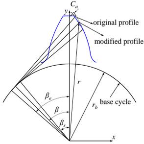
**Fig. 1.** The schematic of tip relief.
