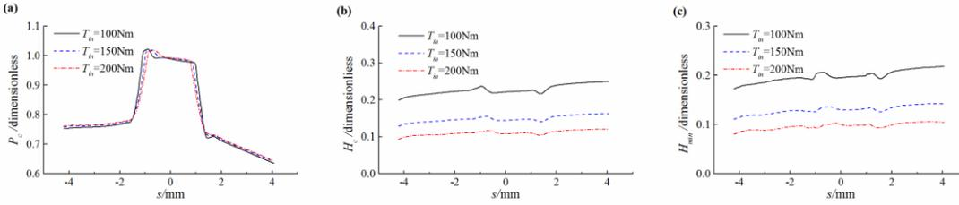
**Fig.5.** Effects of applied torque on (a) dimensionless central pressure, (b) dimensionless central film thickness and (c) dimensionless minimum film thickness.
